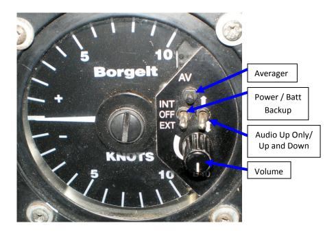
The Borgelt B40 vario is a simple to operate and understand instrument. It has a number of simple features to help give the pilot the needed information.
