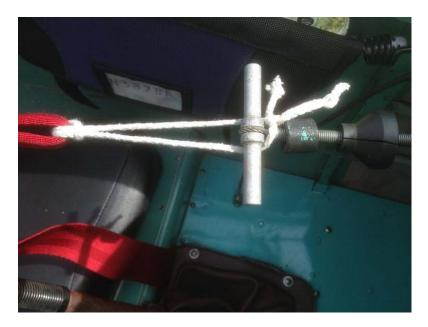
With the strap adjusted close to its shortest possible setting, this will hold the spoilers fully open.
